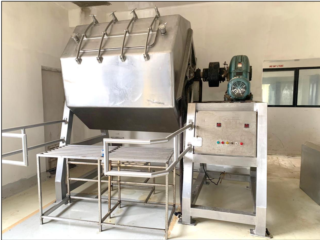
Blender Machine for Dry Granules Mixer
