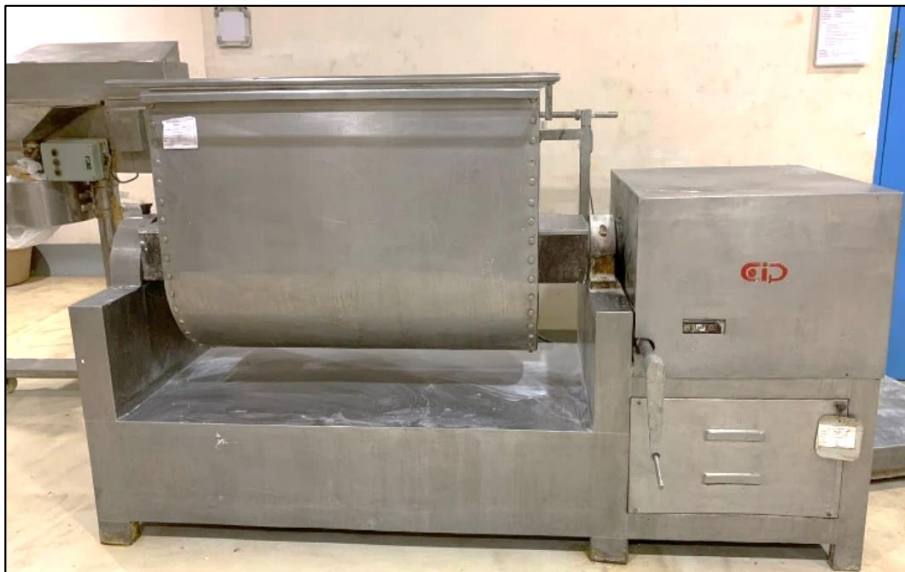
Mass Mixer Machine Use for Powder Mixer
